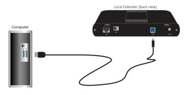
Power the Local Extender with the included 24V 1A AC adapter and tighten the locking ring.
